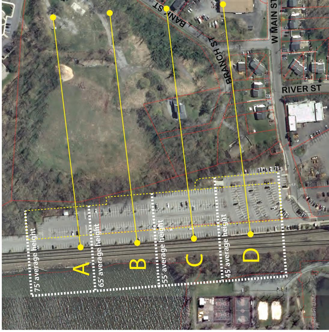
Profile Section Cuts & Building Height Areas
